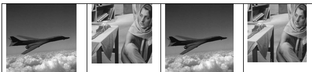
Figure 4. (a) Airplane image ( 512 \times 512 ), (b) Original Barbara Secret image ( 433 \times 433 ) (c) Stego airplane image after embedding Barbara image, and (d) Recover Barbara image.
